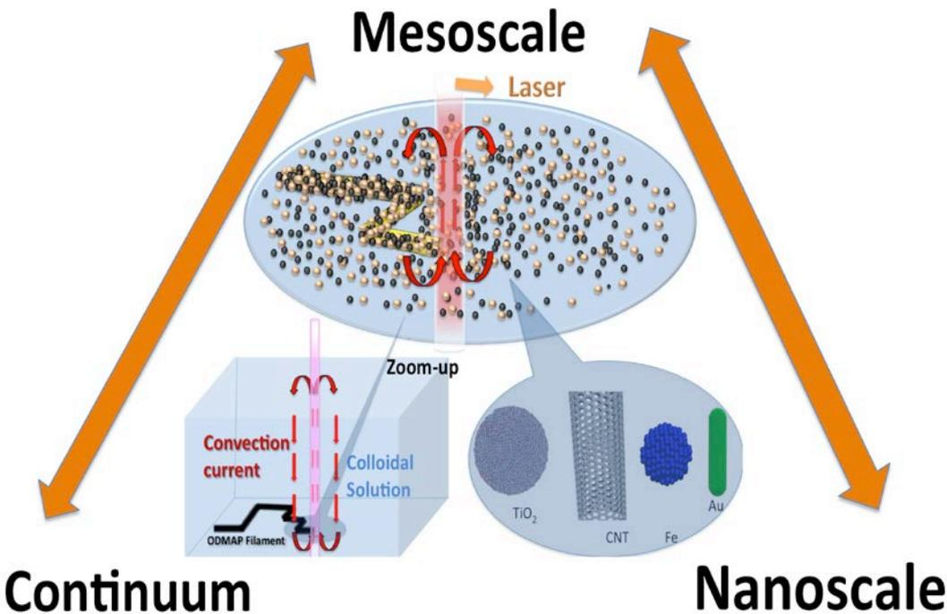
*Optically directed mesoscale assembly and patterning (ODMAP) of electrically conductive organic-inorganic hybrid structures on glass substrates*
