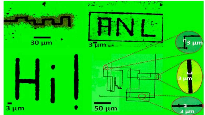
Examples of optically directed patterning of 2-D mesoscale structures comprised of gold and carbon NPs. Such organic-inorganic hybrid structures have relatively high conductivities of  $\sim 430$  S/cm, significantly better than current devices based on organic structures
