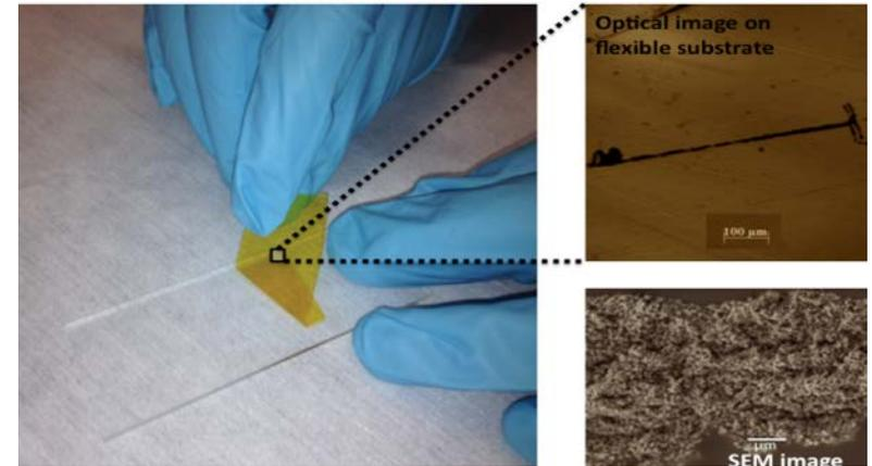
ODMAP structures comprised of Si and Au nanoparticles on a flexible substrate
