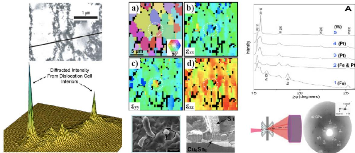
**FIGURE 2.** Applications of x-ray Laue diffraction 3D microscopy. Left: dislocation microstructure and the variation of the local long-range internal stresses in strained single-crystal copper. Middle: local strain gradients induced Sn whisker growth. Crystallographic orientation (a) and strain tensor (b, c, d) maps of the Sn grains near the whisker root are shown. Right: submicron-scale single-crystal x-ray diffraction studies in polycrystalline samples at ultra-high pressures.
