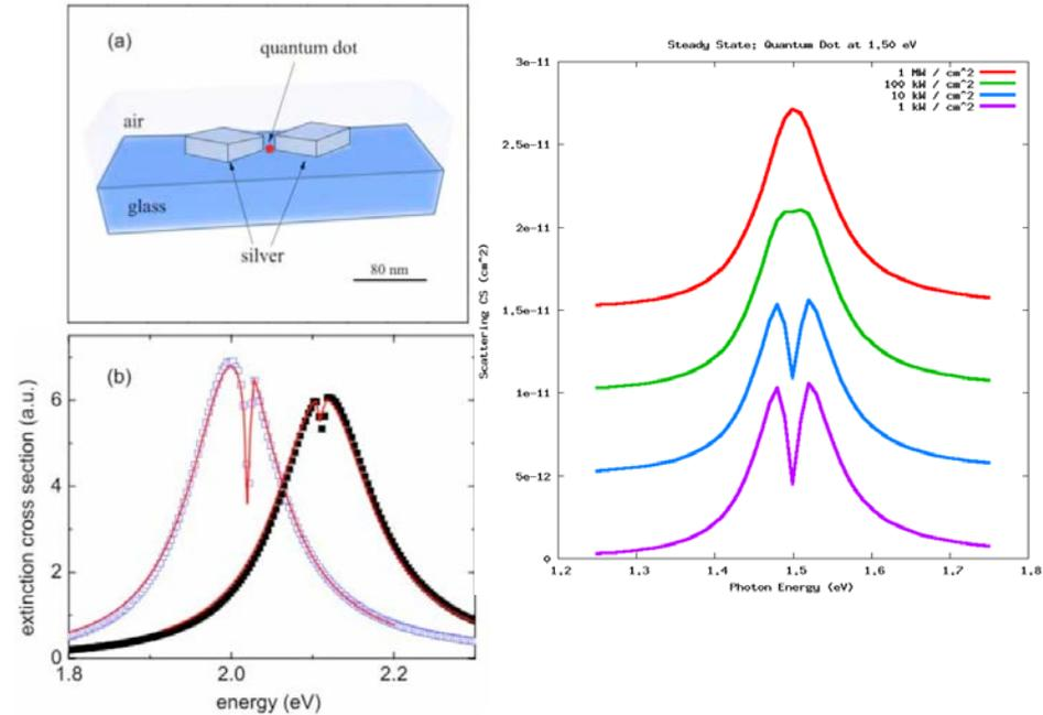
Coupled plasmonic-quantum dot nanoparticle systems (left) show unique optical transparencies (X. Wu, S. Gray, and M. Pelton, *Optics Express* **18**, 23633 (2010)). These transparencies are predicted to respond nonlinearly to incident light (right), thus opening a means for an optically controlled switch of photon flow from the nanoscale to the mesoscale.
