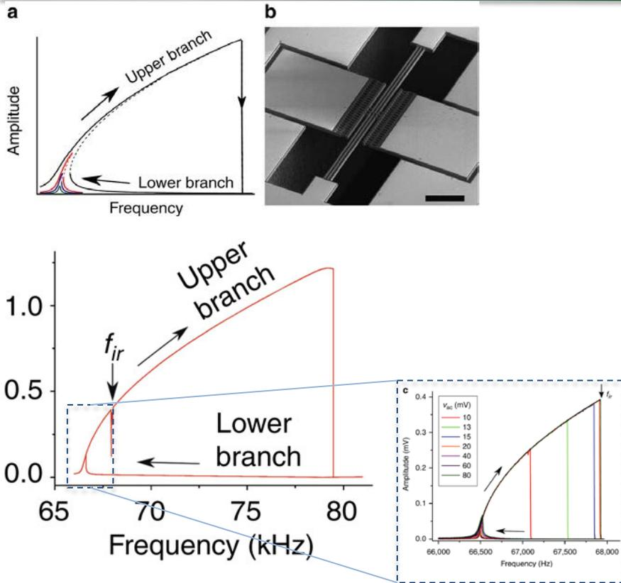
Frequency stabilization in nonlinear nano-mechanical oscillator via coupling to different vibrational modes through internal resonance. This result demonstrates that very low-frequency noise performance is possible in the nonlinear regime.
