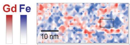
Figure 2: Scanning transmission electron microscopy image illustrating the nm-scale compositional heterogeneity of an FeCoGd alloy. Color scales denote deviation from the average (figure courtesy of Hermann Durr, SLAC).
