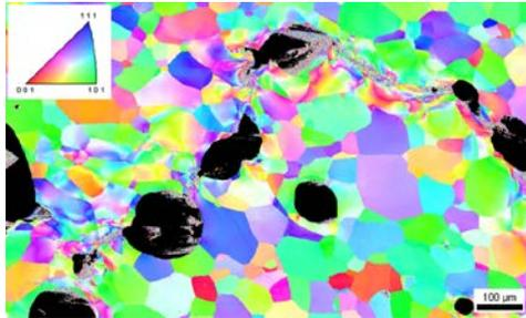
Pores and pore coalescence in dynamically loaded Tantalum
