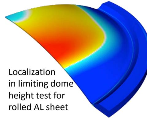
Localization in limiting dome height test for rolled AL sheet
