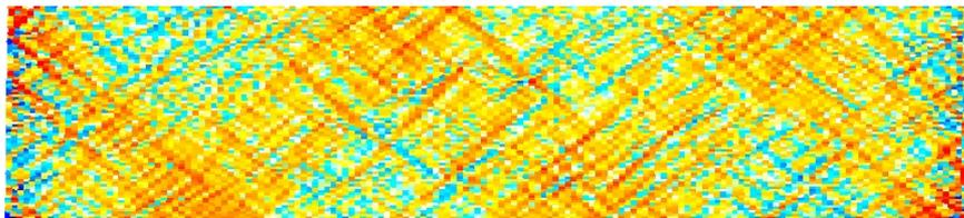
Localization of deformation under plane-strain compression
